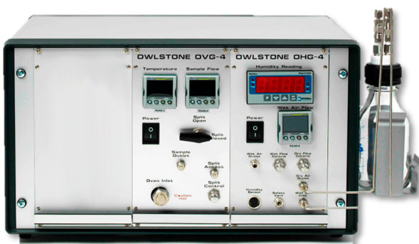
Fig.2. Owlstone vapour generator (OVG) and Owlstone humidity generator (OHG).
