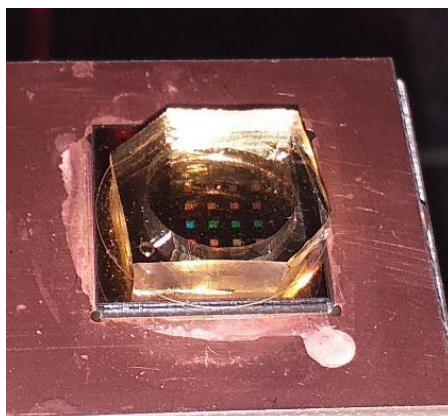
Fig.1 Photograph of the optical sensor (1.5cmx1.5cm). The grating area is 500µmx500µm. PDMS container and lid is also shown.
