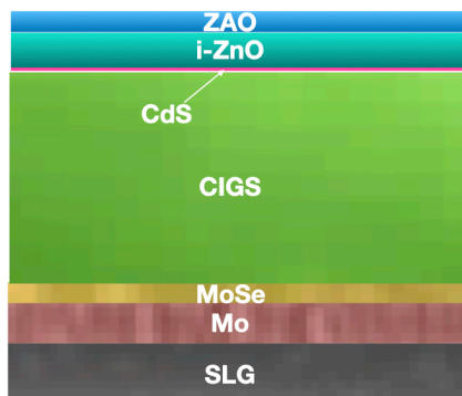
Fig. 1. CIGS device structure.
