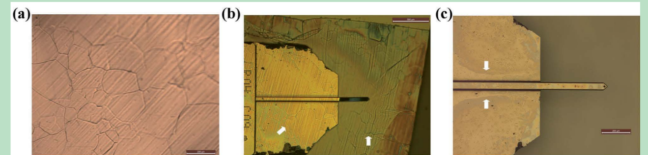
Fig.1. Optical images of the (a) fresh GSL on copper, (b) PMMA/GSL stack transferred on the tip, and (c) graphene-coated tip after PMMA removal. The cantilever of the tip tends to bend due to the weight of the PMMA (b), and it recovers its initial position after removing it (c). The scale bars for (a), (b) and (c) are 200 \mu\text{m} , 500 \mu\text{m} and 200 \mu\text{m} , respectively.
